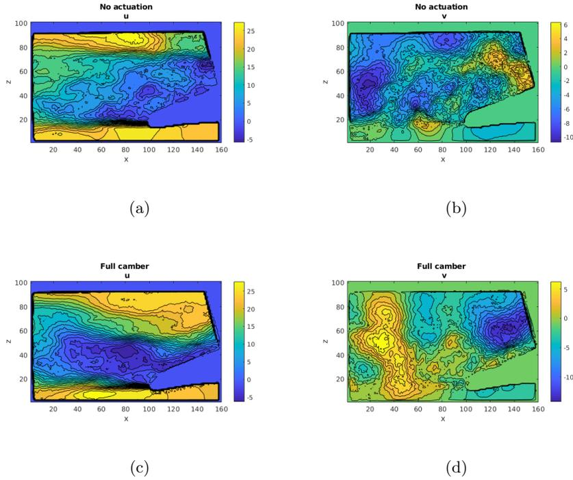
Fig. 11: Reconstruction of the flow using POD modes: (a) and (b) show the two velocity components of the static case ( $t = 1.4$  seconds); (c) and (d) correspond to the full camber position ( $t = 2.36$  seconds).
