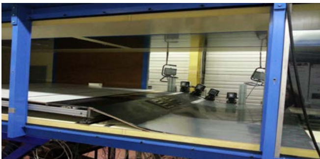
Fig. 2: Photography of the ramp model. The flow is coming from the left
